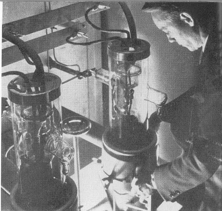
This unusual photograph shows Joseph A. Chambers, Technical Supervisor of 500,000-watt WLW, placing in position one of the twenty great 100,000-watt water-cooled tubes used in the WLW transmitter.
