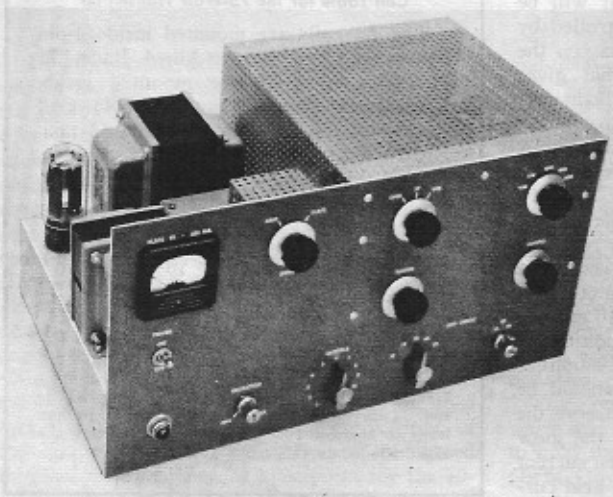
Fig. 6-43—This 75-watt crystal-controlled transmitter has provision for the addition of v.f.o. control. A 6AG7 oscillator drives a 6DQ5 amplifier on 80 through 15 meters.
